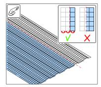
Rods can be cut to length using a grinder, metal saw or pipe cutter. The cut-off side must be equipped with a new insert, which can be ordered separately.
